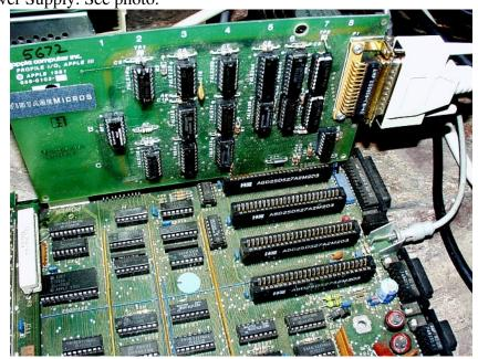
Connect the cable between the interface card and the Profile.
